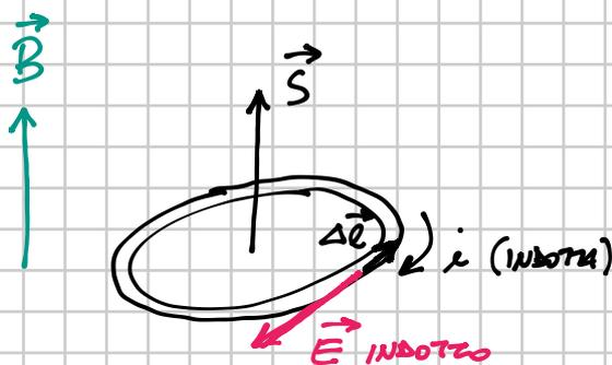
$$\oint_{\mathcal{L}} (\vec{E}) = - \frac{\Delta \Phi(\vec{B})}{\Delta t} \quad \text{IN MODULO} \quad \left| \oint_{\mathcal{L}} (\vec{E}) \right| = \left| \frac{\Delta \Phi(\vec{B})}{\Delta t} \right|$$
