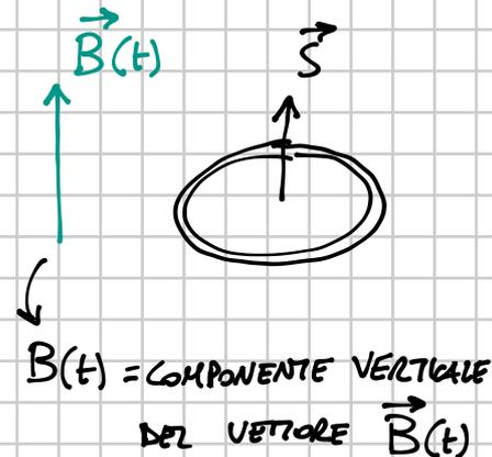
$$\left| \Gamma_{\mathcal{L}}(\vec{E}) \right| = \left| \frac{d\Phi(\vec{B})}{dt} \right|$$
